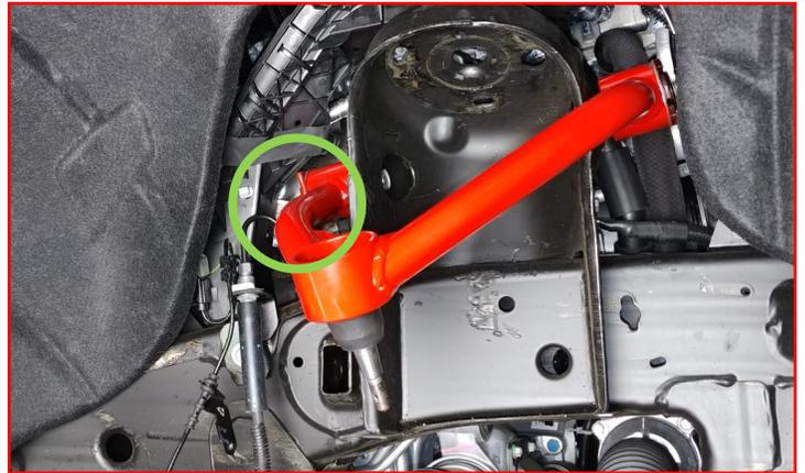
With the upper control arm bolts in place, install the supplied **laser cut washers, the supplied M14 washers and nuts**.
