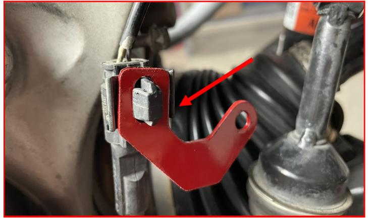
Install the **Brake Pad Sensor Relocation Bracket** on to the knuckle using factory hardware.
