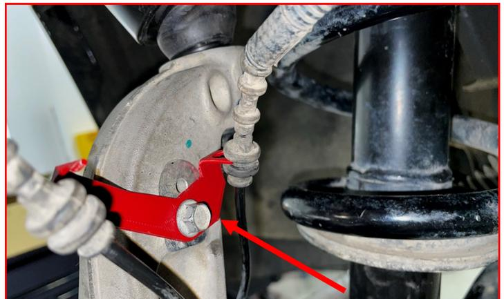
Remove the factory brake pad sensor bracket from the knuckle.
