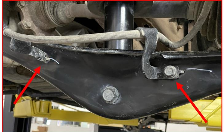
Support the lower control arm with a suitable jack. Peel back the fender liner to remove the three (3) **upper strut bolts**.
