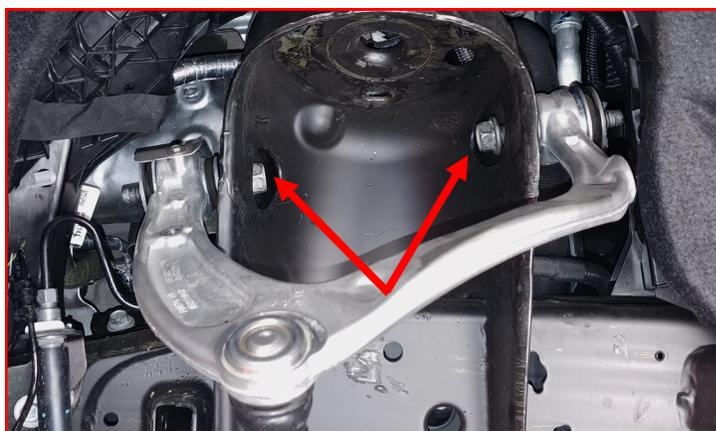
Mark the studs 1.125" from top of strut, use appropriate cutting tool to trim stud to the proper height.
