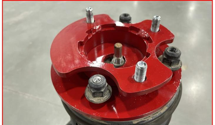
Using the supplied **M10-1.25 Serrated Flange nuts**, install the rear strut assembly into the strut tower.
