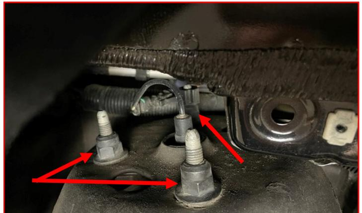
Remove the **lower knuckle bolt**. Lower the jack enough to allow for the knuckle to release from the lower control arm.
