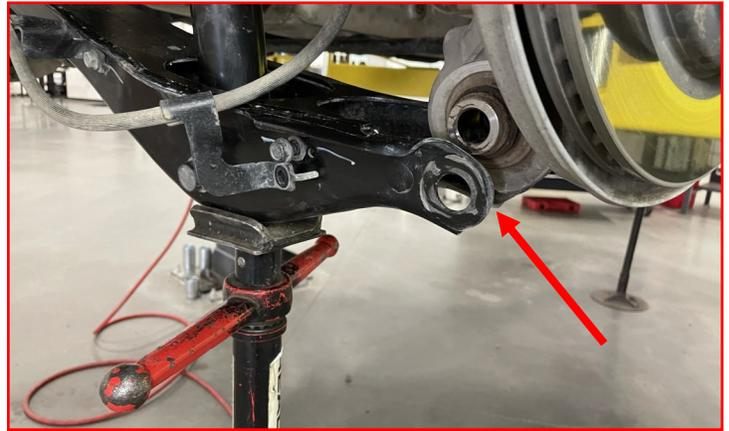
Remove the **strut nut and bolt**. Retain factory hardware.
