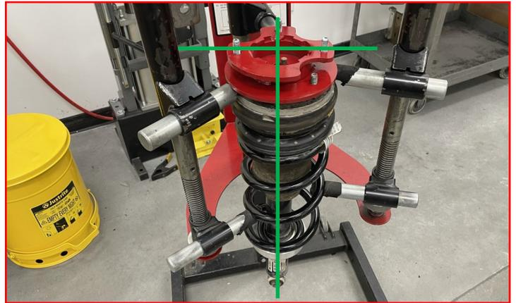
Using factory hardware, install and tighten the **Rear Strut Spacer** onto the strut.
