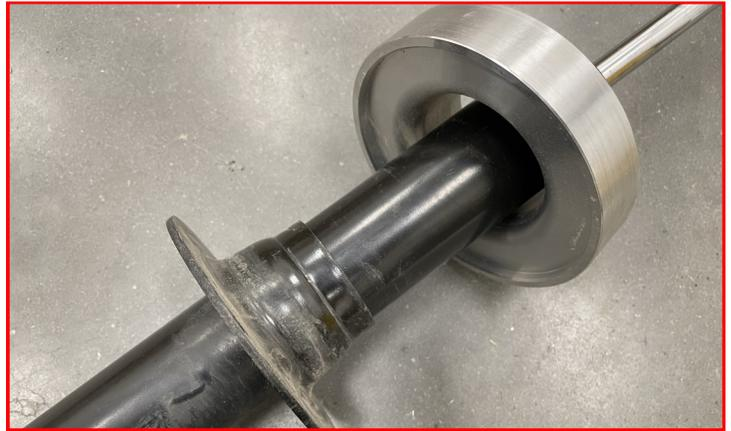
Using the **ReadyLift Rear Strut Spacer** as a guide, align the strut so the lower strut bolt hole is **perpendicular** to the two studs in the **Rear Strut Spacer**.
