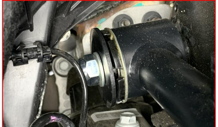
Once upper control arms have been properly torqued, install completed strut assembly. Install with supplied **M10 nuts**.
