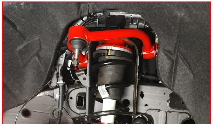
Remove the **lower nut clip** from the strut and discard.
