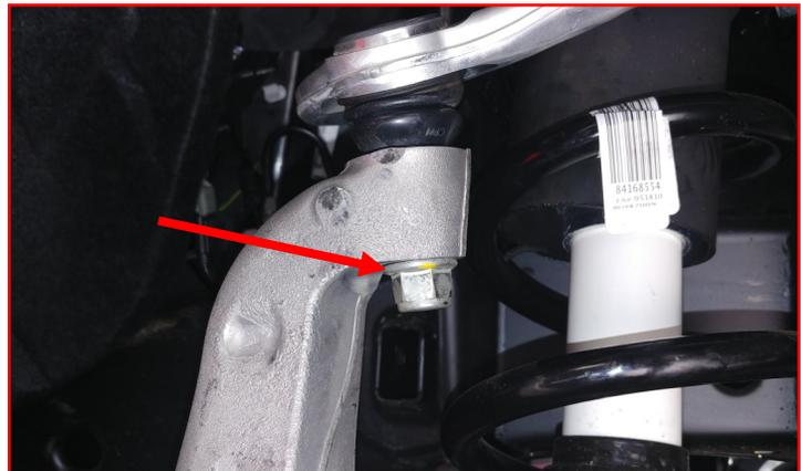
Support the lower control arm with a suitable jack. Remove the **lower strut mounting bolt** from the lower control arm. Discard factory bolts.
