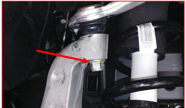
Support the lower control arm with a suitable jack. Remove the **lower strut mounting bolt** from the lower control arm. Retain the factory bolts.
