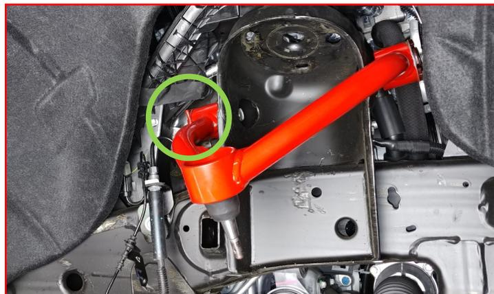
With the upper control arm bolts in place, install the supplied **laser cut washers**, the **factory nuts** and a drop of thread locker.
