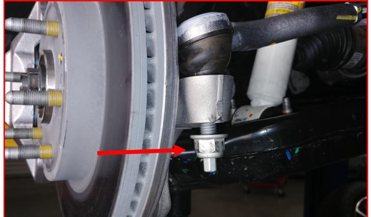
Remove the **ABS sensor harness and the brake-line bracket** from the knuckle and hang out of the way. Retain factory hardware.
