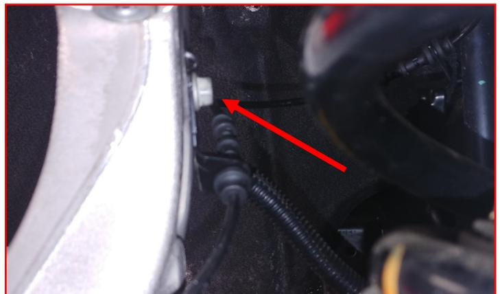
Install the **ABS bracket** to the Upper Control Arm using supplied **1/4" nut and washer**.
