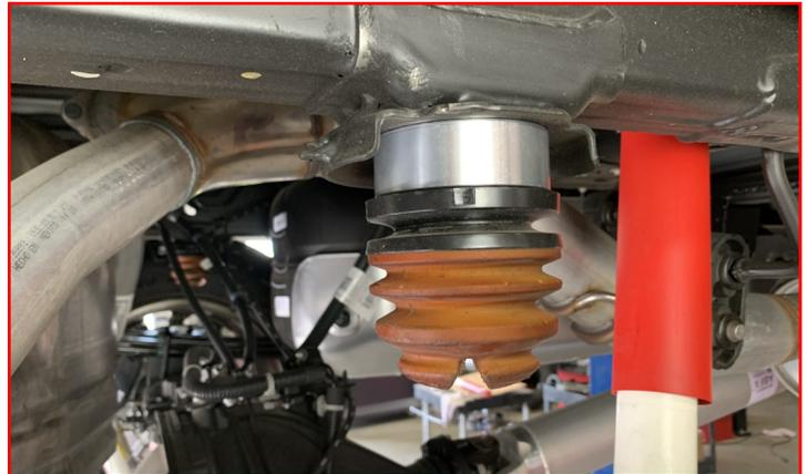
Remove factory bolt that attaches the rear jounce stop to frame and discard the bolt. Install **rear jounce stop extension** between frame rail and jounce stop using supplied M10 Bolts and washers.
