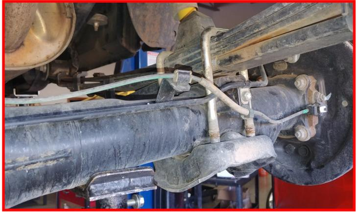
Remove the u-bolts of the side you are working on and discard.
