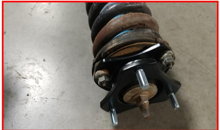
Install the completed strut assembly to the frame using the provided hardware. Do not tighten at this time.
