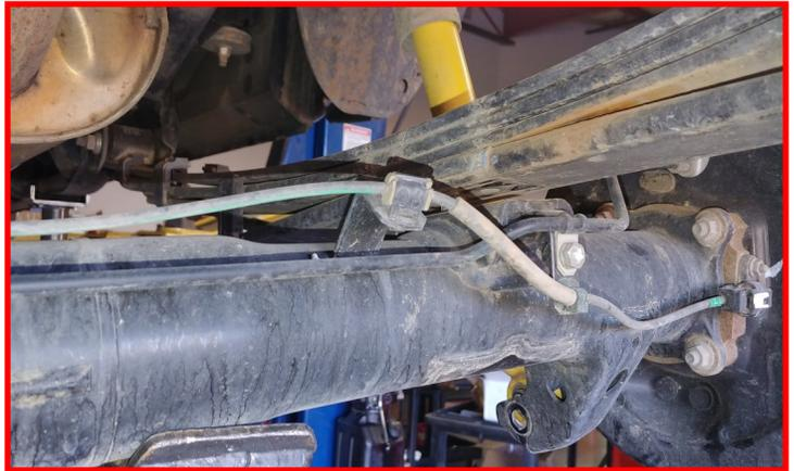
Lower the axle low enough to install the ReadyLIFT block. If the block is tapered, make sure the small end of the block is towards the front of the vehicle. Raise the axle while lining up the center pins. Install the provided u-bolts and hardware. Do not tighten fully, leave loose so that you can repeat the steps for the opposite side. Repeat all steps above regarding the block install.
