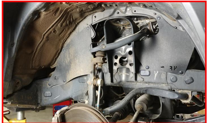
Install the ReadyLIFT strut extension to the strut using the **factory hardware**. Torque to **30 ft-lbs**.
