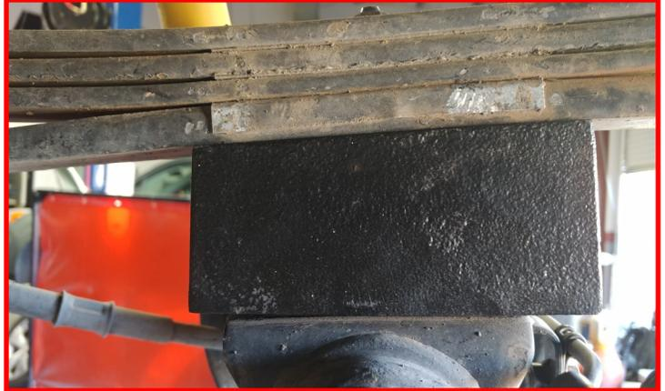
Install the shock lower hardware. Do not tighten at this time. Install the wheels and lower the vehicle to the ground. Jounce the vehicle to settle the suspension to the new ride height. Torque the lower shock hardware to **45 ft-lbs**, and the u-bolts to **110 ft-lbs**.
