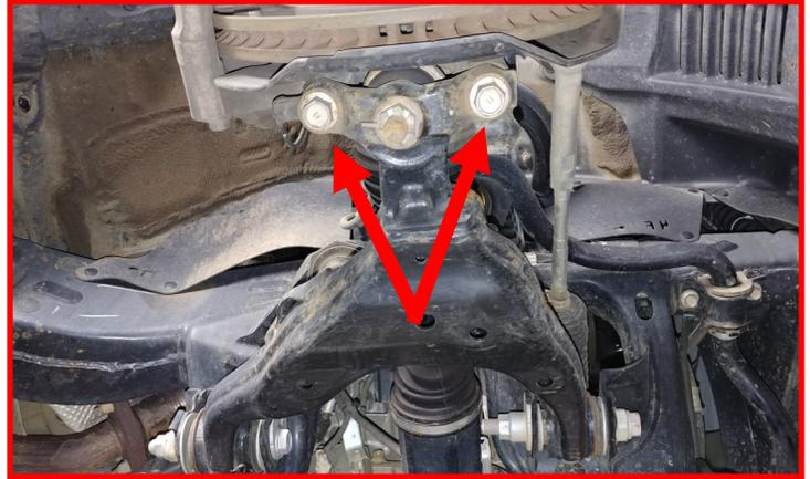
Loosen but do not remove the lower control arm cam bolts. Let the control arm swing down and hang out of the way.
