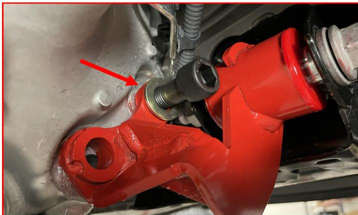
Install the **factory hardware (driver side differential bolt)** into the lower hole.
