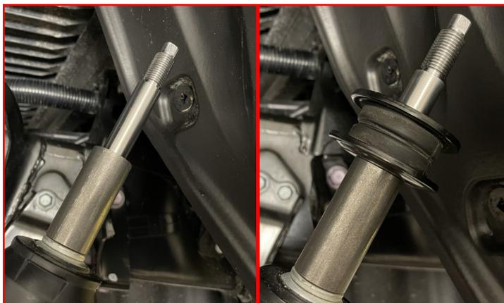
Install the **upper factory shock bushing** and **nut**.
