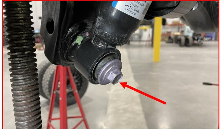
Remove the **upper shock nut** and bushing.
