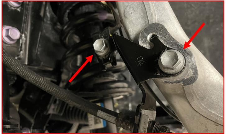
Using **factory hardware**, attach the ABS sensor wire at the bottom of the knuckle.
