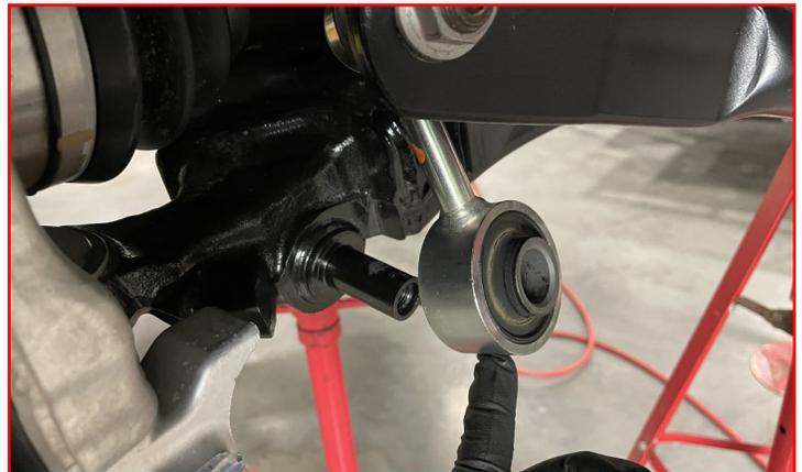
Remove the **ABS wire bracket** on the upper control arm.
