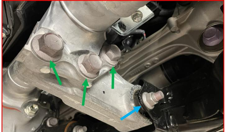
Remove the **two bolts** holding the **driver side bracket** to the differential.
