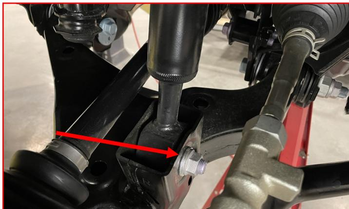
Remove the four (4) **upper strut bolts**.
