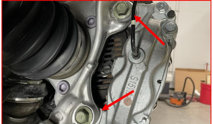
Remove the upper ball joint **retaining clip** by pushing in on the clip nub.
