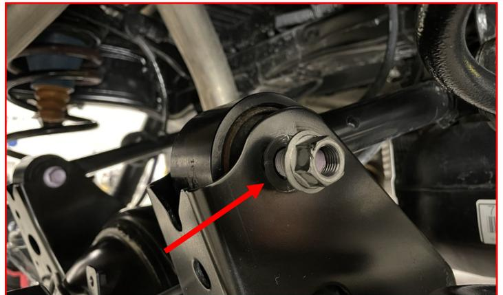
Remove the **lower factory strut bushing** from the shock.
