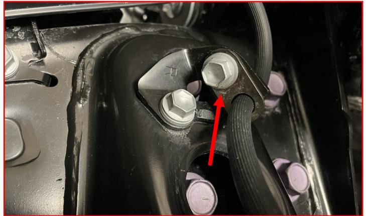
Remove both **screws** retaining the ABS wire to the middle of the knuckle.
