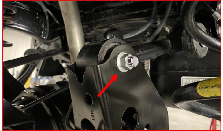
Loosen but **DO NOT** remove the **lower control nut** at the axle.
