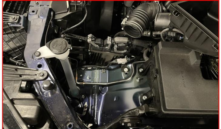
Remove the three (3) **bolts** holding the accumulator to the body.
