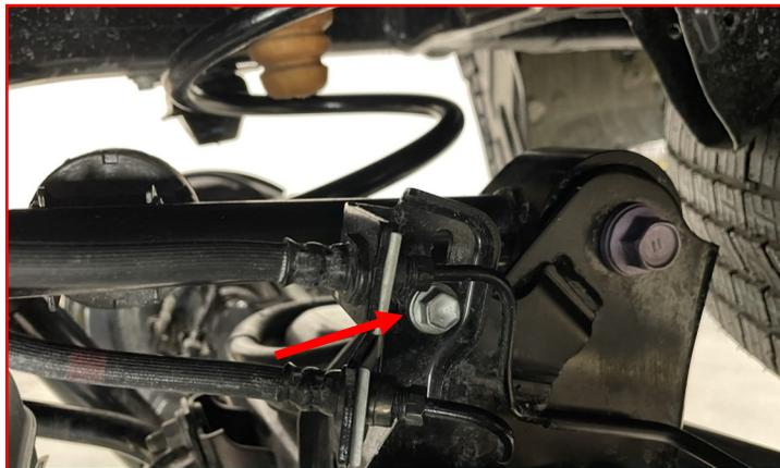
Install the end link onto the frame using **factory hardware**.
