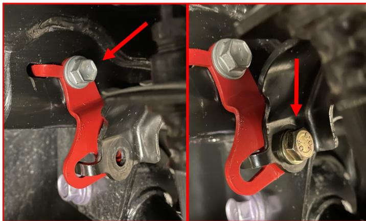
Install the bracket (one on each side) holding the brake line to the axle using **factory hardware**.
