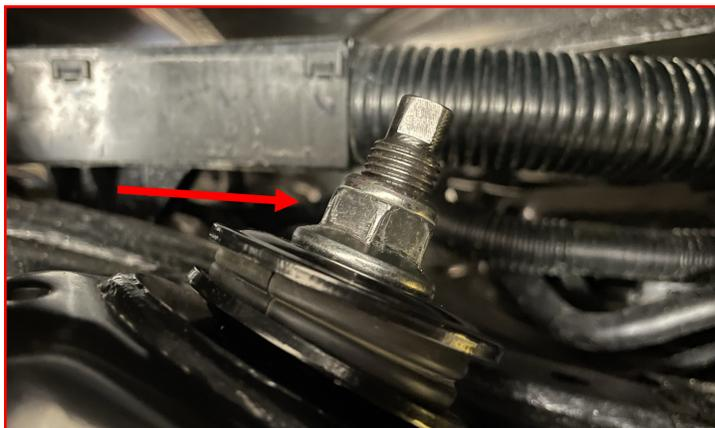
Torque the **lower shock bolt** to 60 ft-lbs.
