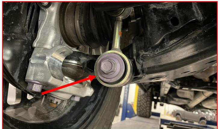
Torque the sway bar bracket **factory hardware** to **80 ft-lbs.**
