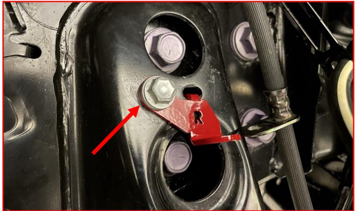
Attach the brake line to the **brake line bracket** using **factory hardware** and the supplied **M8-1.25 locking nut** and **M8 washer**.
