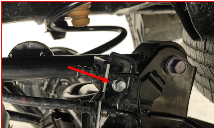
Remove the **end link nut** and let the end link hang out of the way.
