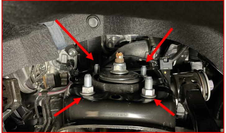
Loosen but **DO NOT** remove **inner control arm nuts**.
