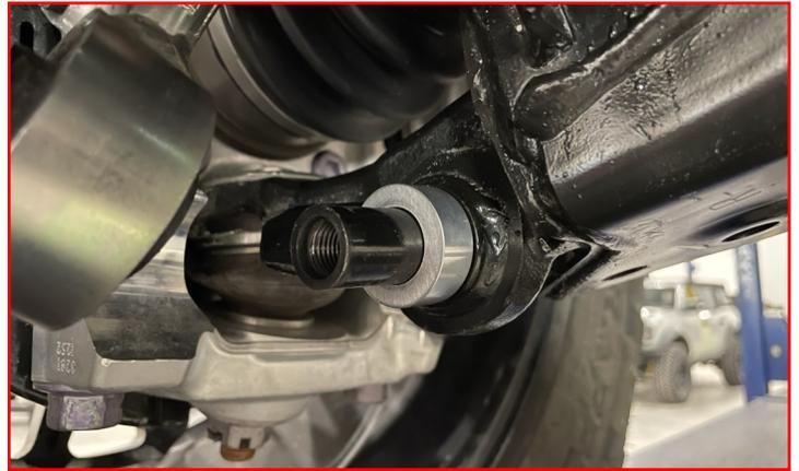
Torque the sway bar end link **factory hardware** to **80 ft-lbs.**
