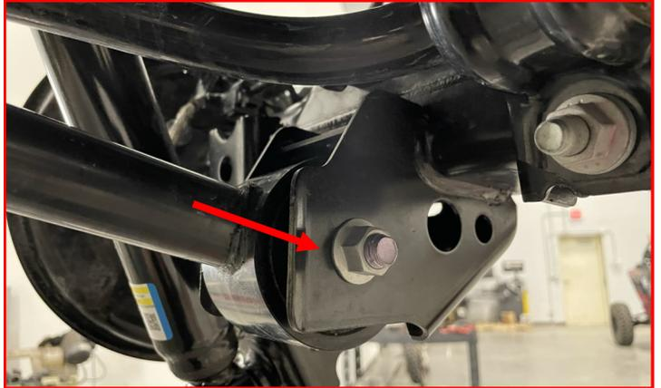
Loosen but **DO NOT** remove the **lower shock bolt**.
