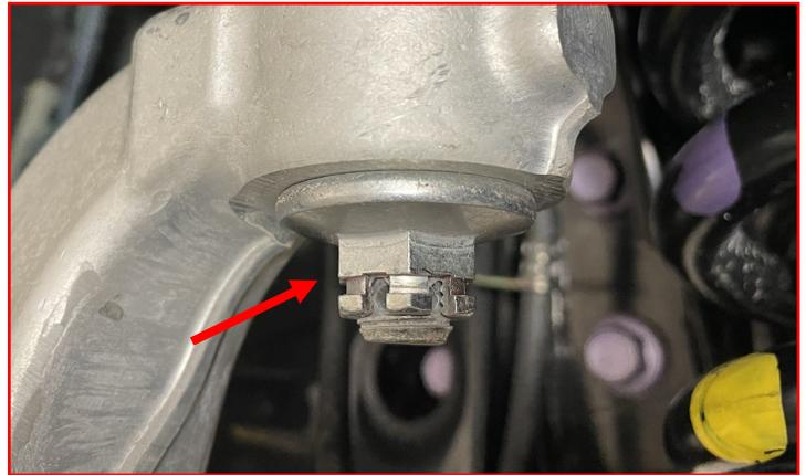
Use the appropriate tool to release the taper on the upper ball joint.
