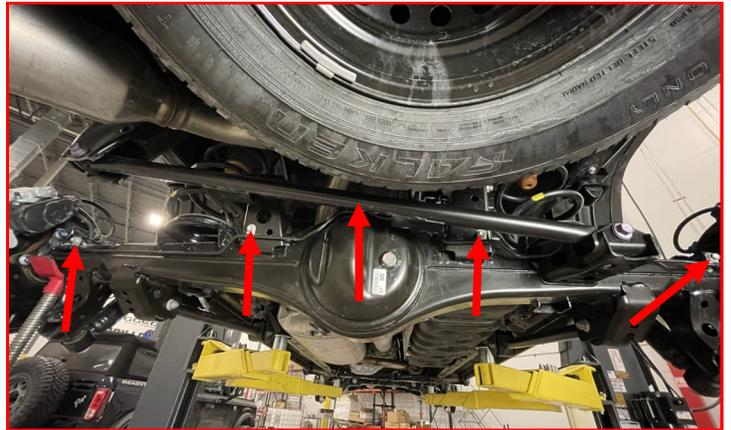
Install the **rear brake line spacer** between the brake line and the axle using the **factory bolt** (one on each side) holding the brake line to the axle.
