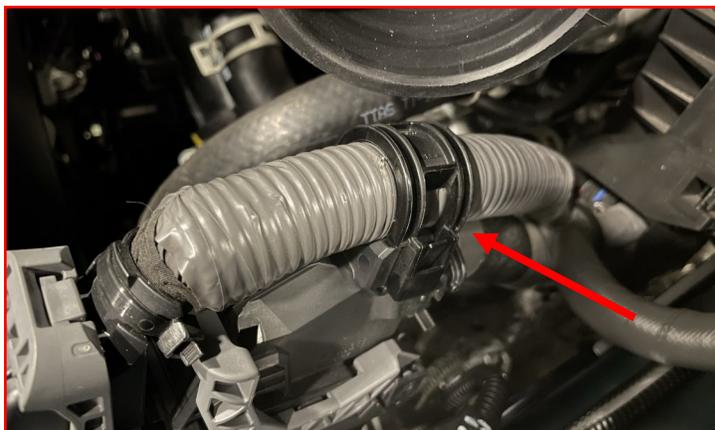
Plug the left most plug into the accumulator and lock it in place by closing the handle to the left.
