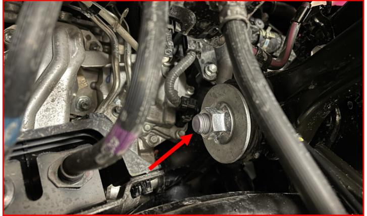
Remove the **upper control arm bolt** and remove the **upper control arm**.
