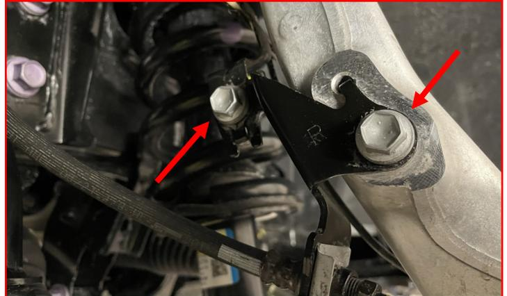
Remove the **ABS wire bracket** at the bottom of the knuckle.
