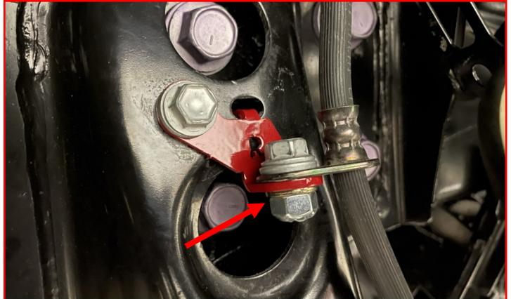
Attach the upper control arm ABS wire bracket to the upper control arm stud using the supplied **M8 locking nut** and **M8 washer**.
