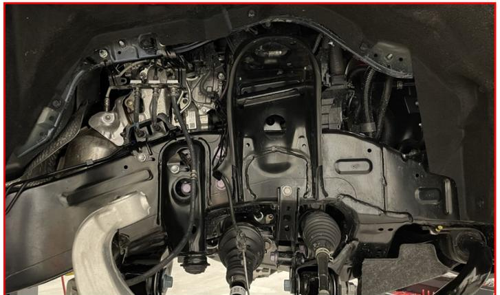
Install ReadyLift **front strut spacer** onto the strut using **factory hardware**.
