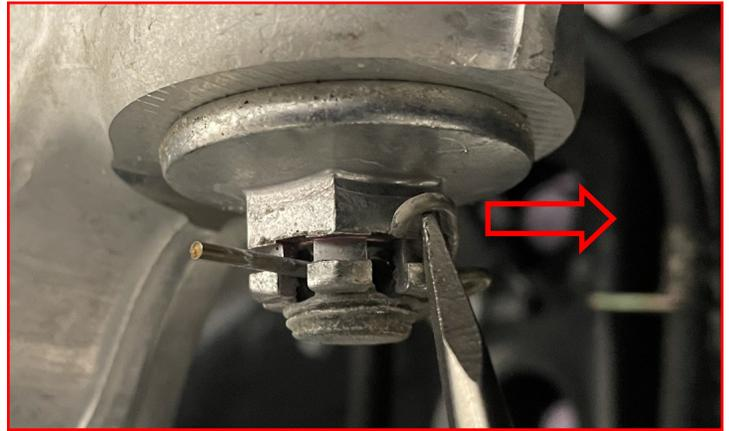
Loosen but **DO NOT** remove the **upper ball joint nut**.
