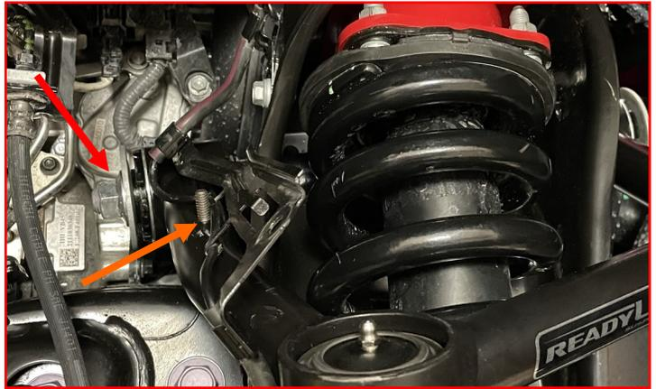
Lower the upper control enough to insert the ball joint stud into the knuckle using the supplied **M12-1.75 flange nut**.
