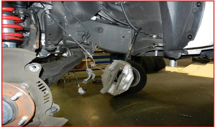
Remove the upper ball joint safety clip and nut. Strike the ball joint boss with a dead blow hammer to dislodge the taper.
