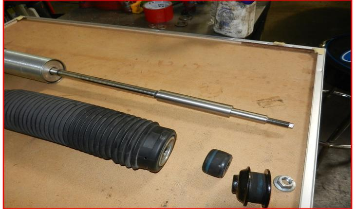
Stretch the boot until it fits over the shock body and install the hose clamp to hold boot in place.
