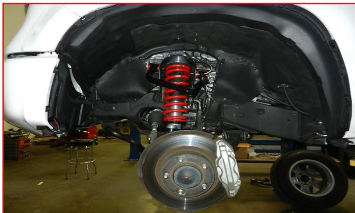
Install the brake line bracket to the ReadyLIFT control arm using the **supplied nut and washer**. Torque to **5 ft-lbs**. Install the outer tie rod end to the knuckle using **factory hardware**. Install the cotter pin. Torque to **65 ft-lbs**. Install the ABS sensor and wire harness to the knuckle using the **factory hardware**. Torque to **5 ft-lbs**.
