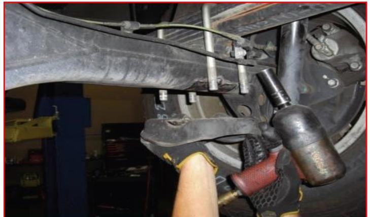
Install the parking brake brackets to the ReadyLIFT extensions using **5/16" x 1" bolts, washers, and c-lock nuts**. Install completed assembly to the axle using **factory hardware**. Torque all hardware to **5 ft-lbs**. Install the ABS bracket to the charcoal canister using the factory hardware. Torque to **5-ft-lbs**.
