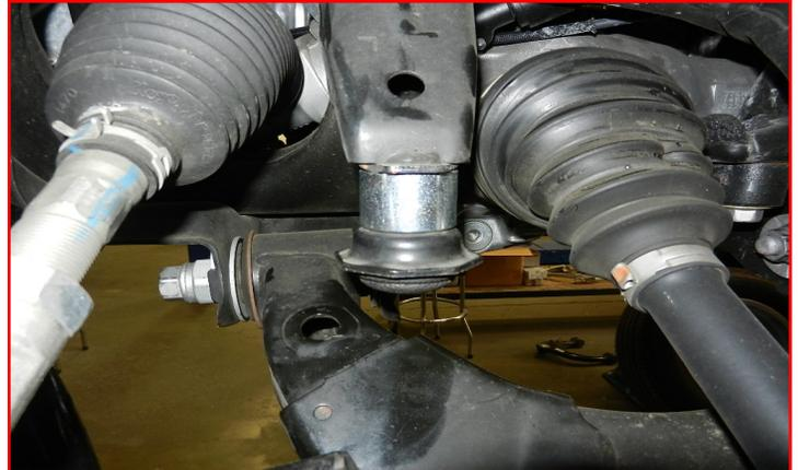
Notch the lower control arm strut pocket as shown using a suitable cutting device. Sand any burs off the cut edge. Paint the cut area with a quality rust preventative paint.
