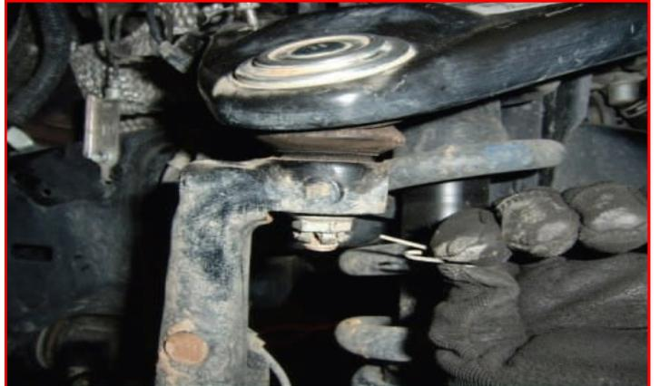
Remove the front splash guards from the frame for access to the upper control arm bolt.
