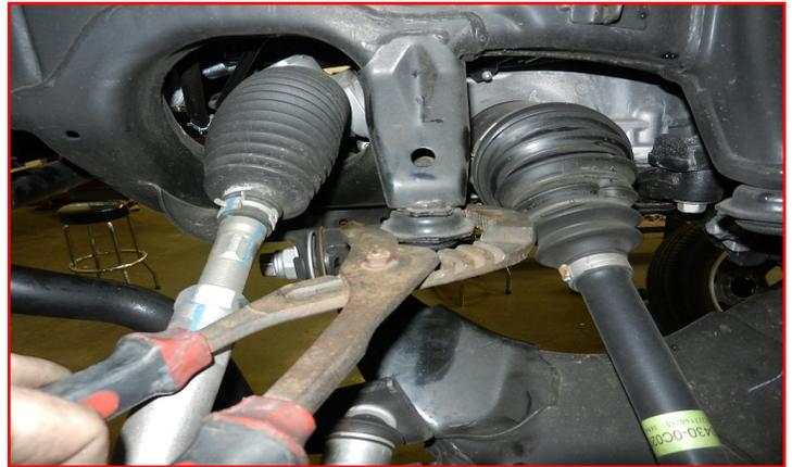
Install the ReadyLIFT bump stop extensions onto the frame and then the factory bump stops to the extensions.
