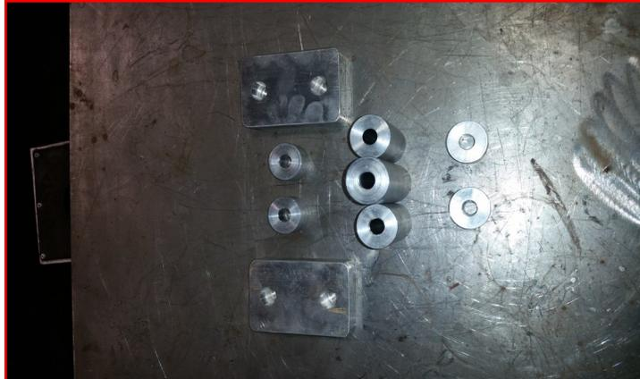
There are 9 billet spacers used on the pro skid plate. 2 rectangular, 4 small round, 2 medium round, and 1 large round. Picture shows placement for the spacers.
