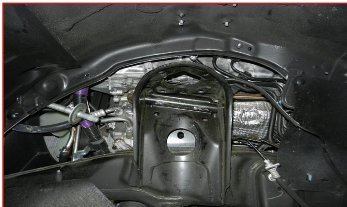
Install the bushings and sleeves into the ReadyLIFT control arms using the supplied grease packet if you have the non forged arms. Install the ReadyLIFT upper control arm to the frame using the factory hardware, and supplied large washer to the inside edge of the control arms. Do not tighten at this time.
