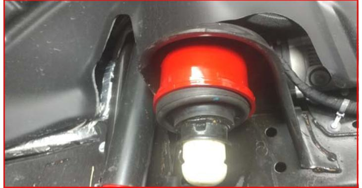
Insert the front bump stop **3/8" x 1.75" Allen bolt** into the front bump stop. Insert the front bump stop into the coil spring. Install the coil spring and bump stop at the same time to the frame and axle.
