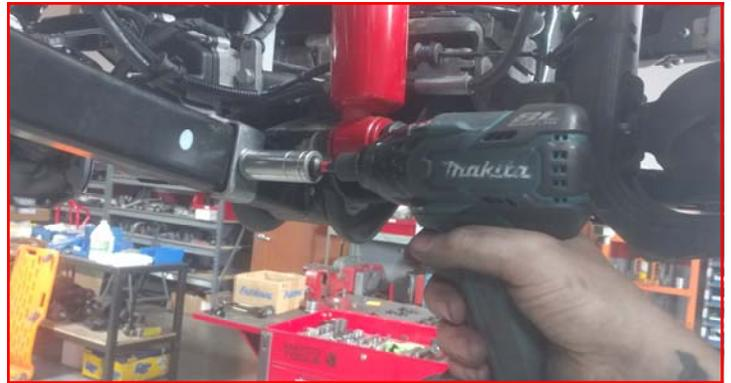
Remove the front sway bar end links from the axle. Save the hardware.
