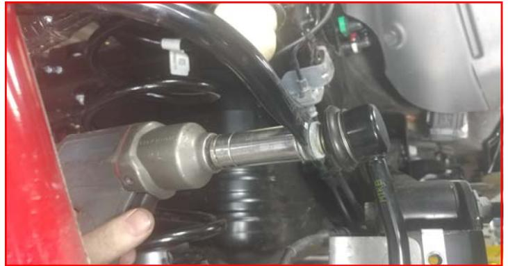
Loosen but do not remove the rear upper control arms at the axle and frame.
