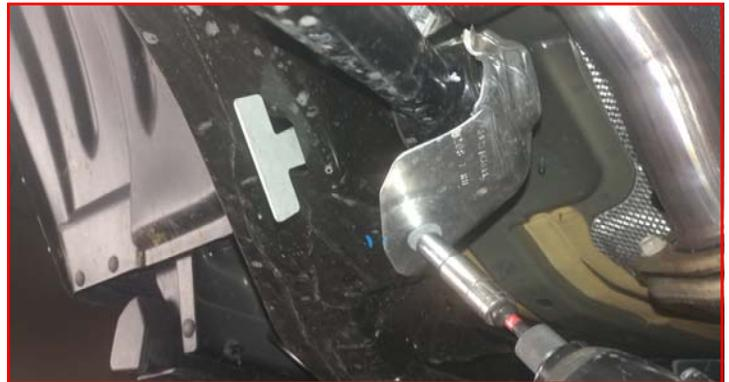
Gently bend the heat shield out of the way and loosen but do not remove the front upper control arm bolts.
