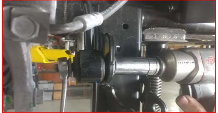
Remove the rear upper sway bar end link from the sway bar.
