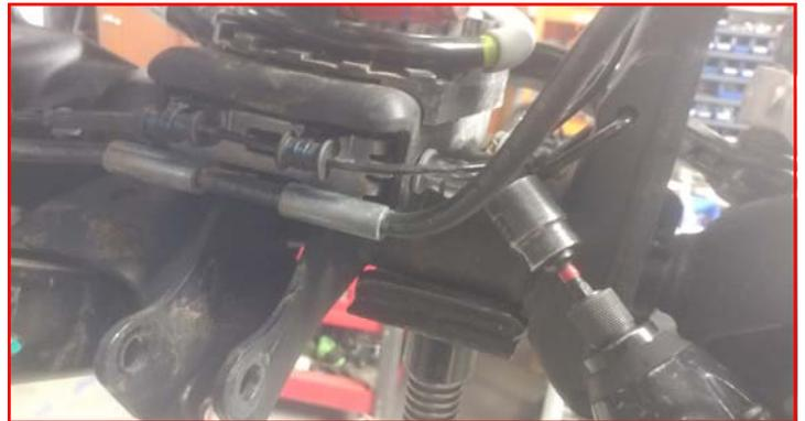
Install the provided **3/8" serrated flange nut** to the **3/8" Allen bolt** from the under side of the spring perch. Torque to **35 ft-lbs**.
