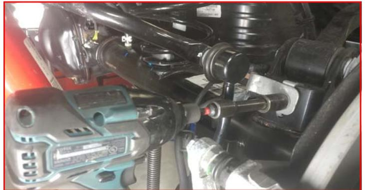
Remove the rear lower shock from the axle.
