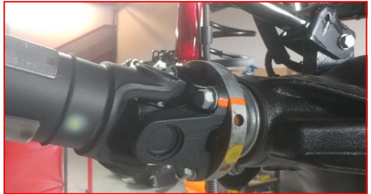
Remove the drive shaft from differential.
