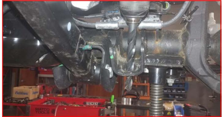
Install the ReadyLIFT front shock extension using provided **1/2" x 1.25" bolt, washers, and nut**. Use the factory bolt to line up the holes while tightening the **1/2" hardware**. Once tight, remove the factory hardware.
