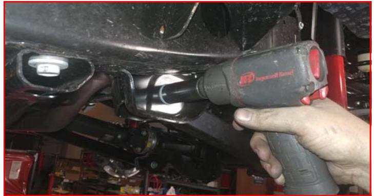
Remove the lower heat shield bolt from the front upper control arm pocket at the frame.
