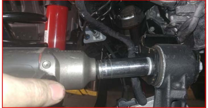
Mark the drive shaft to pinion flange for reinstallation later.
