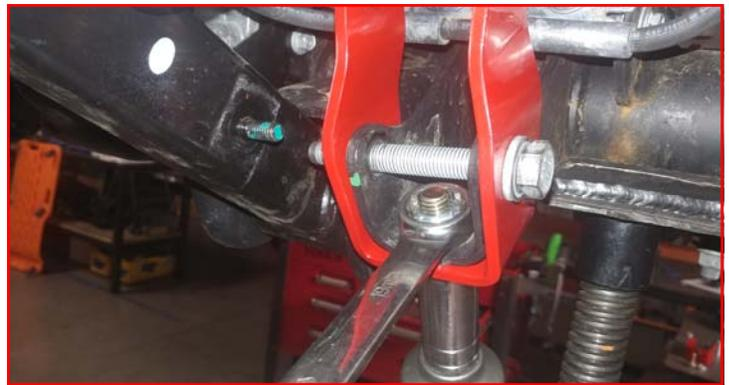
Install the ReadyLIFT **crush sleeve and the factory shock bolt** in the lower hole. Do not tighten at this time. Install the lower shock using the provided **1/2" x 2.75" bolt, washers and nut**. Do not fully tighten at this time.
