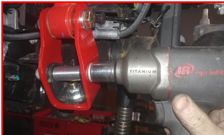
Install the brake line brackets to the lower control arm and frame rail using the **factory hardware**. Torque to **5 ft-lbs**.
