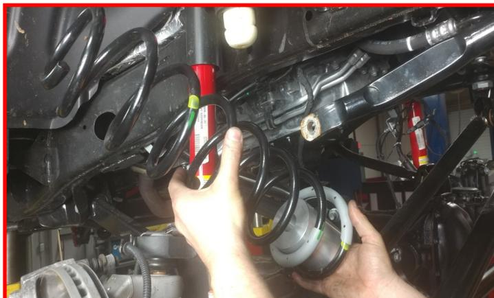
Install the coil spring and bump stop at the same time to the frame and axle making sure to clock the spring so that the dead end of the coil sits in the lock on the axle pad. Raise the axle enough to hold the springs in place.
