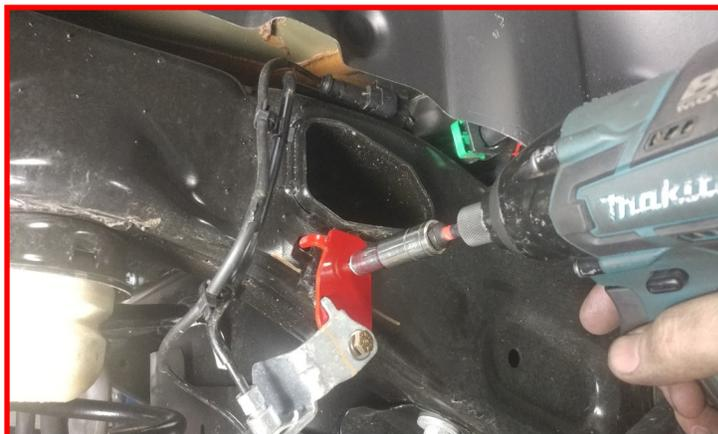
Install the ReadyLIFT rear bump stops to the axle using the provided **1/4" x .75" bolts, washers, and nuts**. Torque to **5 ft-lbs**. (69-6835 kit number bump stops do not have R logo and are only 2.5" tall)
