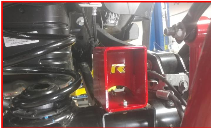
Install the ReadyLIFT e-brake cable to the body using the **factory hardware** and the factory e-brake bracket to the ReadyLIFT bracket using the provided **1/4" x .75" bolt, washers, and nut**. Torque all to **5 ft-lbs**.
