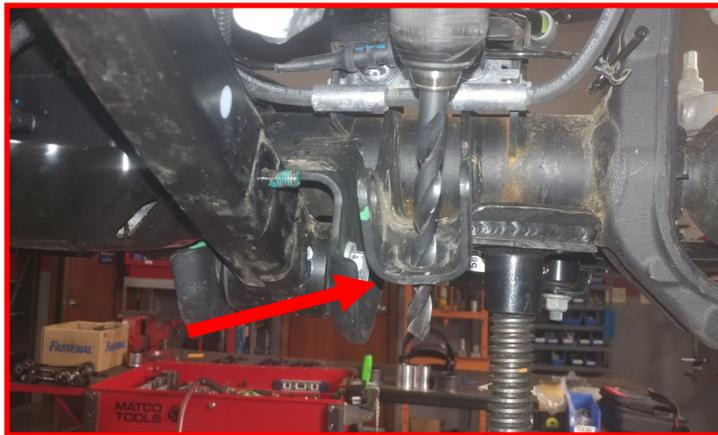
Install the ReadyLIFT front shock extension using provided **1/2" x 1.25" bolt, washers, and nut**. Use the factory hardware to line up the holes while tightening the **1/2" hardware**. Once tight, remove the factory hardware.
