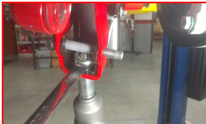
Install the ReadyLIFT **crush sleeve and the factory hardware** in the lower hole. Do not tighten at this time. Install the lower shock using the provided **1/2" x 2.75" bolt, washers and nut**. Do not fully tighten at this time.
