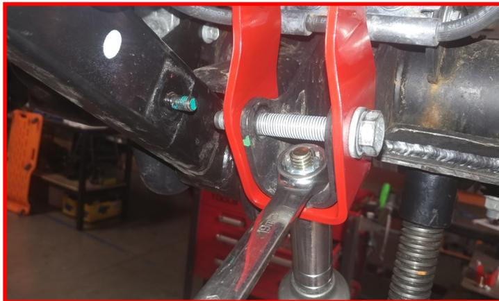
Install the ReadyLIFT **crush sleeve and the factory shock bolt** in the lower hole. Do not tighten at this time. Install the lower shock using the provided **1/2" x 2.75" bolt, washers and nut**. Do not fully tighten at this time.
