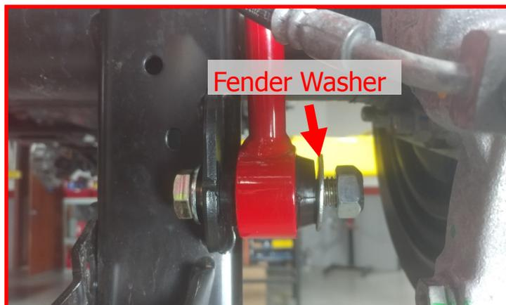
Install the ReadyLIFT rear shock extension using provided **1/2" x 1.25" bolt, washers, and nut**. Use the factory bolt to line up the holes while tightening the 1/2" hardware. Once tight, remove the factory hardware.
