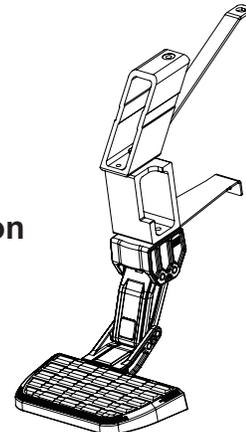
Assemble Frame mount(4) to Lateral mount(3) with Bracket(6) using supplied M8 Flange bolts(13). Do not tighten.
