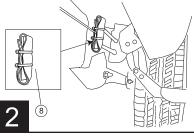
On some models that do not utilize this guide rubber tape (8) is included. Wrap tape around bracket.
