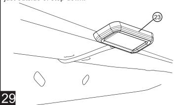
Using supplied butt connectors, connect the lamp wires. Red to Red, Black to Black. Once Crimped use heat gun to shrink tube. Close and wrap conduit with electrical tape. Secure all loose wires with cable ties. Pull lamp wires upward to avoid any wire
