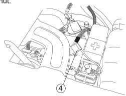
Attach ground lead to negative battery pole.
