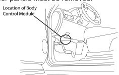
Vehicles that do not have the front door ajar signal wires in the pink connector of the BCM must have the front door panels removed in order to access the front door ajar signal wires. For these and all Hybrid models go to step 20.
