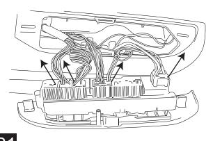
To remove door panel, first pry back tab on door lock to remove then pry off plastic covers by handle and door latch. Remove the 3 door bolts and then remove door panel by prying loose all panel fasteners.
