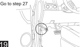
Remove plastic trim on door near mirror attachment. Then carefully pry up window/ door lock switch plate.
