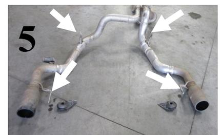
1. Lubricate all hangers, rubber isolators, bolts and nuts.
