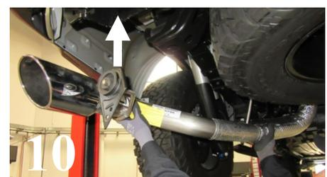
**WARNING:** Use extreme caution during installation. Torque all fasteners according to manufacturer's torque values and tightening sequence. **DO NOT** use air impact tools to tighten fasteners on Borla Performance Exhaust Systems. Use of such tools may result in bent flanges or gasket contact areas leading to exhaust leaks.
