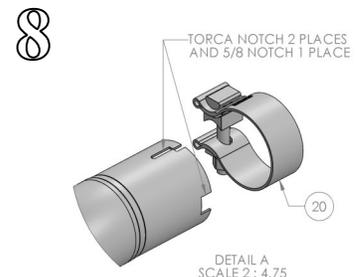
**WARNING:** Use extreme caution during installation. Torque all fasteners according to manufacturer's torque values and tightening sequence. **DO NOT** use air impact tools to tighten fasteners on Borla Performance Exhaust Systems. Use of such tools may result in bent flanges or gasket contact areas leading to exhaust leaks.
