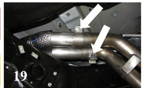
5. Reinstall the OE hanger adjacent to the front muffler pipe. Carefully lift assembly inserting hangers into the rubber isolators and **Muffler Assembly** inlets into the OE front pipe. (See Figs. 15-16)
