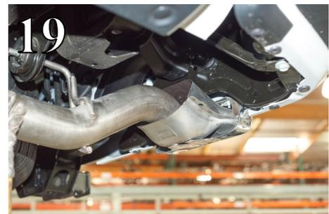
18. Reinstall the stock rubber isolators to hang the Borla tailpipes.
