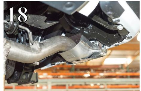
9. Place a clamp on the **Cross Over Tube** and connect it to the **Y-Pipe Assembly** (Fig. 16). Do not tighten the clamp.
