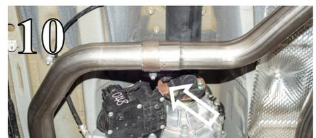
**WARNING:** Use extreme caution during installation. Torque all fasteners according to manufacturer's torque values and tightening sequence. **DO NOT** use air impact tools to tighten fasteners on Borla Performance Exhaust Systems. Use of such tools may result in bent flanges or gasket contact areas leading to exhaust leaks.
