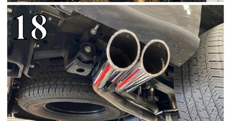
**WARNING:** Use extreme caution during installation. Torque all fasteners according to manufacturer's torque values and tightening sequence. **DO NOT** use air impact tools to tighten fasteners on Borla Performance Exhaust Systems. Use of such tools may result in bent flanges or gasket contact areas leading to exhaust leaks.
