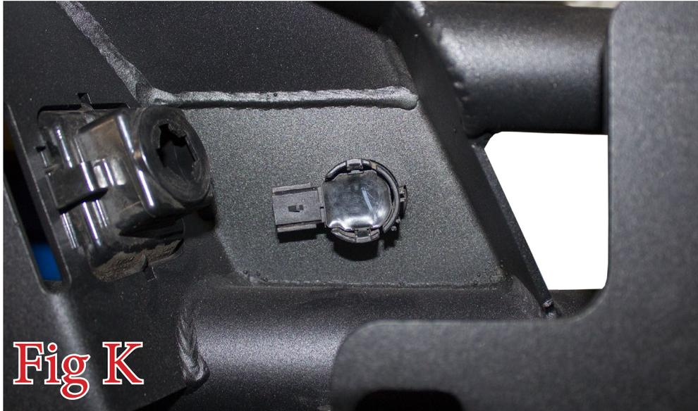
14. Install the trailer plug onto your new bumper. Do this by pressing it into its precut hole until it clicks into place. (Fig L)
