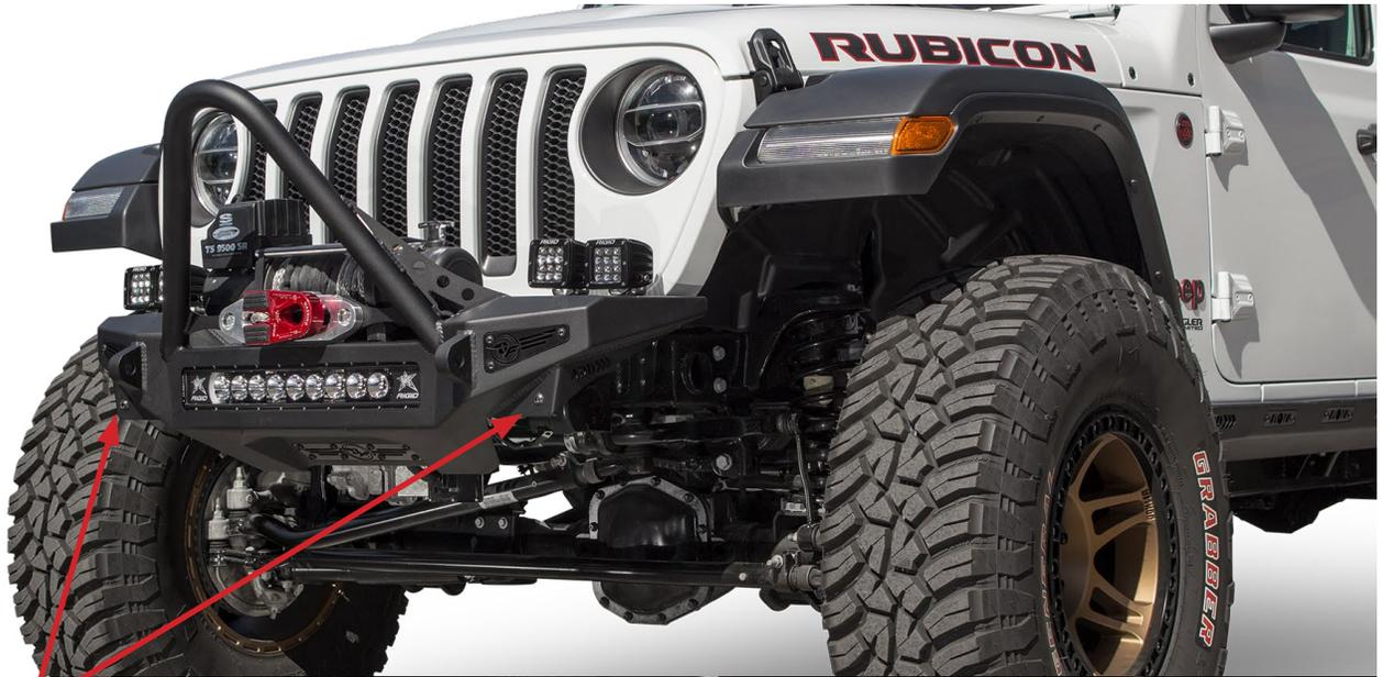
Use 1/2" Bolts on these holes. Install 3/8" Bolts from the back side of the frame horn for the rest of the bolts.
