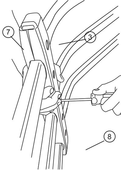
**NOTE:** Do not over tighten as this may strip out. Fastener will reach a noticeable stopping point.
