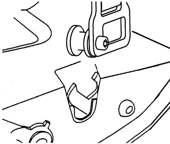
NOTE: Ensure that buckles are properly inserted into latches by pulling on the straps after both buckles have been inserted.
