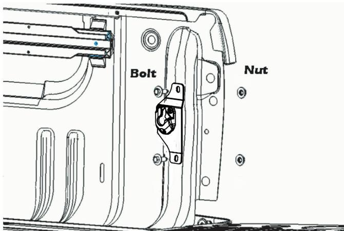
Place Mounting Bracket aligned with top hole. Allow bracket to hang vertically. Mark (Center Punch) location of lower hole using the bracket slot as a template. Remove bracket. Drill hole with 1/8" drill bit then drill out hole with 21/64" drill bit. Use file to remove burrs. Apply primer to edge of hole. Allow primer to dry.
