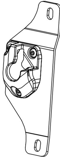
Use the M5 bolts and nuts to fasten the Quick Mount Bracket to the mounting bracket. Apply thread locker to the tip of the M5 bolt. Torque to 8 ft. lbs. Allow 10 minutes to dry before handling. (Passenger side shown)
