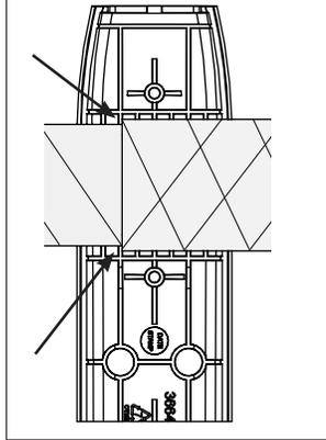
**NOTE:** The inside of the upright is stepped to fit correctly around the small and large diameter tubes.
