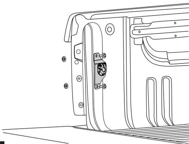
Place Mounting Bracket aligned with top hole. Allow bracket to hang vertically. Mark (Center Punch) location of lower hole using the bracket slot as a template. Remove bracket. Drill hole with 1/8" drill bit then drill out hole with 21/64" drill bit. Use file to remove burrs. Apply primer to edge of hole. Allow primer to dry.
