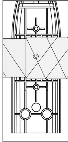
**NOTE:** The inside of the upright is stepped to fit correctly around the small and large diameter tubes.
