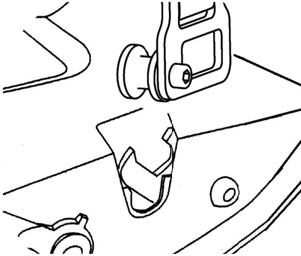
**9** When the BEDXTENDER is at the furthest rear position, push down on the buckle to insert into tailgate latch. Tighten straps. To release, pull tailgate handle.
