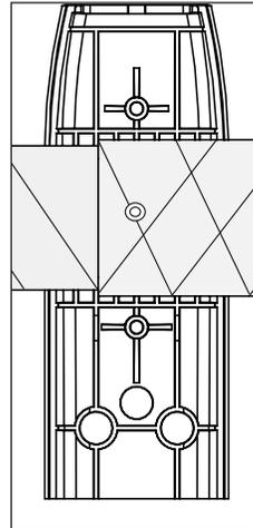
**7** NOTE: The inside of the upright is stepped to fit correctly around the small and large diameter tubes.
