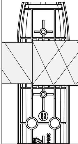
**7** NOTE: The inside of the upright is stepped to fit correctly around the small and large diameter tubes.
