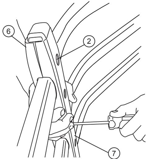
**8** NOTE: Do not over tighten as this may strip out. Fastener will reach a noticeable stopping point.
