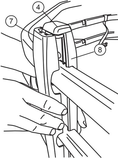
*Upright is not positioned in center of tube joint.*
