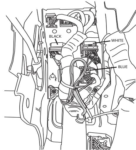
35 **NOTE: Plug reassembly is critical. Lever Arm of plug must be rotated completely locked in the open position to engage properly!**
