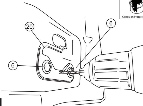
Once hole is drilled insert a piece of string or wire through hole in Reinforcement Plate. Set plate into position.
