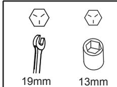
**11** NOTE: Hold Rivet tool with wrench while loosening bolt.
