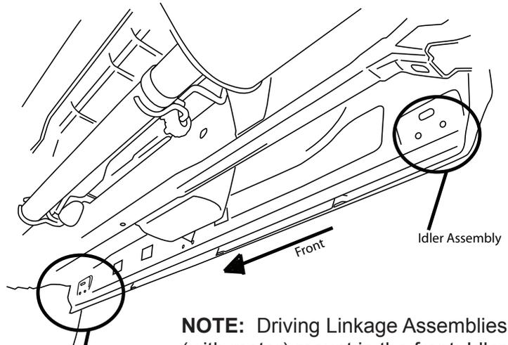
**NOTE:** Driving Linkage Assemblies (with motor) mount in the front; Idler Assemblies mount in the rear.
