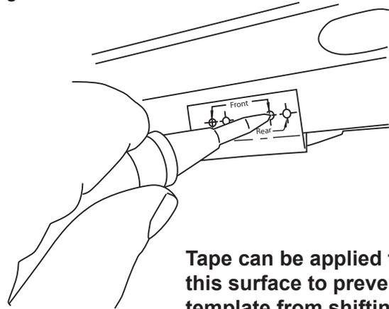
Tape can be applied to this surface to prevent the template from shifting.
