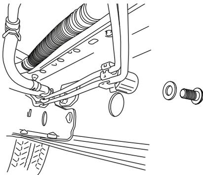
Replace all brake line fasteners.
