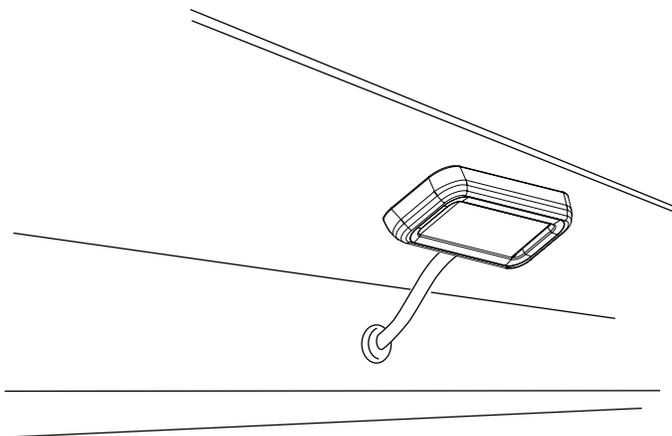
Using supplied butt connectors, connect the lamp wires. Red to Red, Black to Black. Once Crimped use heat gun to shrink tube.
