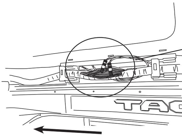
*Carefully open wire harness contained in black plastic split loom*
