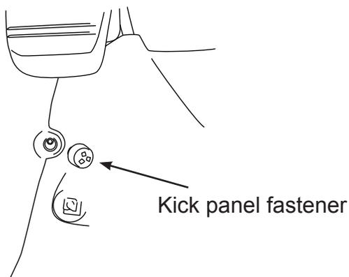
Pull up carpet and locate rubber grommet. Slice the grommet and pass trigger wires from under the vehicle and into the cab.
