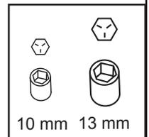
**Torque bolts to 6 ft-lbs / 8 Nm.**
