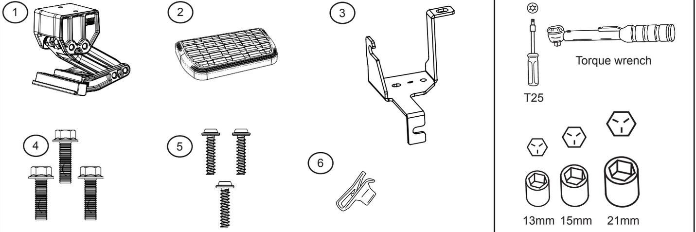
Using a 15mm wrench assemble steel bracket to Linkage assembly. Torque bolts to 20 ft-lbs.
