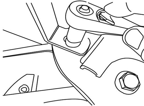
Note: Passenger side bracket will need supplied nut to tighten bracket into place. Use the upper hole. Do not tighten
