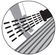
**MAINTENANCE TIPS** - The stepping surface and linkage should be periodically washed with mild soap and water using a soft brush or sponge to dislodge any mud, dirt or accumulated road grime. **In severe driving conditions, pressure washing the linkage is strongly recommended.** Do not apply silicone spray, waxes or protectants like Armor All® to the stepping surfaces.
