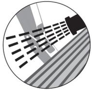
**MAINTENANCE TIPS** - The stepping surface and linkage should be periodically washed with mild soap and water using a soft brush or sponge to dislodge any mud, dirt or accumulated road grime.
