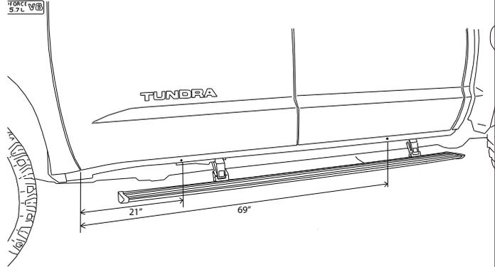
Drill a 9/32" hole through the pinch weld at marked locations. Deburr all holes.
