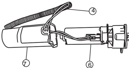
Partially separate the plastic rivet from the pin by bending the pin back and forth. Slide motor cover over motor and insert plastic push pin rivets in mounting holes of motor cover. Drive pin flush with rivet head. Use pliers to ease installation.
