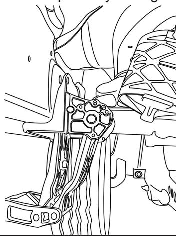
**All Linkages:** Slide linkage over pre threaded bolts. Using a T27 Torx driver start torx bolts and washers. Snug bolts but do not tighten. Replace bolts from step 15 if present.
