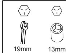
**6** NOTE: Hold Rivet tool with wrench while loosening bolt.
