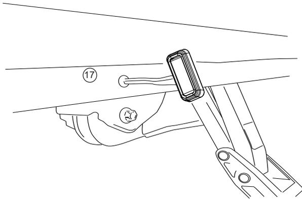
Insert grommet(17) into drilled holes. Insert lamp(10) wires through the grommets. (Silicon lube will help wires slip through grommets.)
