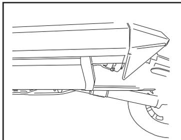
Using a 13mm socket Torque linkage bolts 4x (9) from step 3 to 16 ft-lbs. Next use a 10mm socket, torque linkage spacer bolt 2x (13) from step 6 to 8 ft-lbs. Once linkages are tight cycle board to verify steps deploy under own weight.
