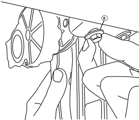
Install provided spacer (17) and M6 bolt (12) into upper mount as shown on both the Drive and Idler linkages. Do not tighten.
