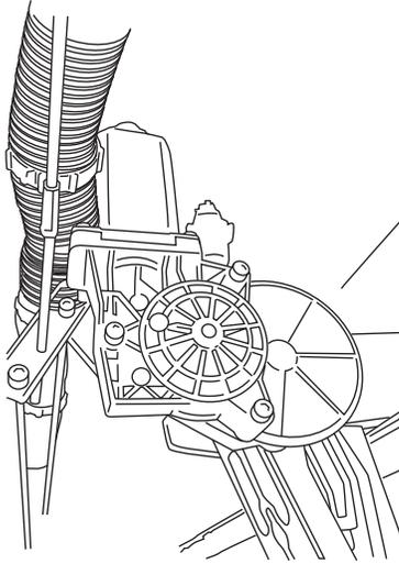
Torque bolts on mounting brackets to 16ft-lbs.
