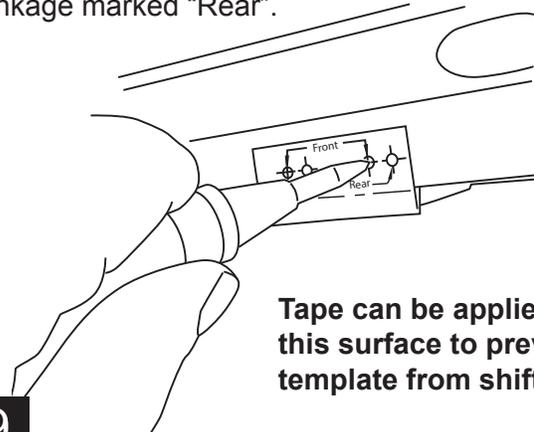
Tape can be applied to this surface to prevent the template from shifting.
