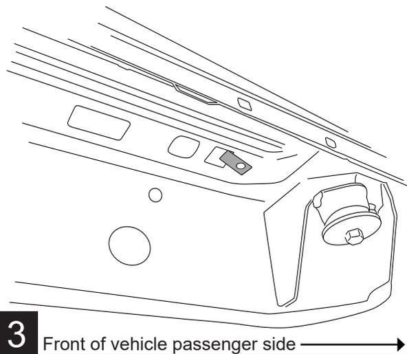
Install Front Drive Linkage assembly. Use button head bolts with washers and Hex flange bolt Torque to 16 ft-lbs. (22N m)
