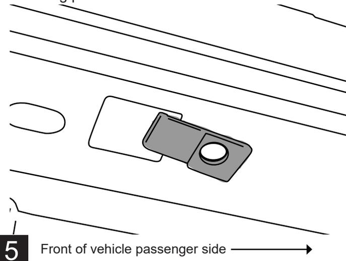
Install Rear Drive Linkage assembly. Use button head bolts with washers and Hex flange bolt Torque to 16 ft-lbs. (22N m). Install light bracket on front side of linkage as in step 4.
