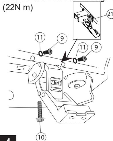
Note: Install light bracket between pinch weld and linkage mount as shown. Install brackets on forward holes of linkage.
