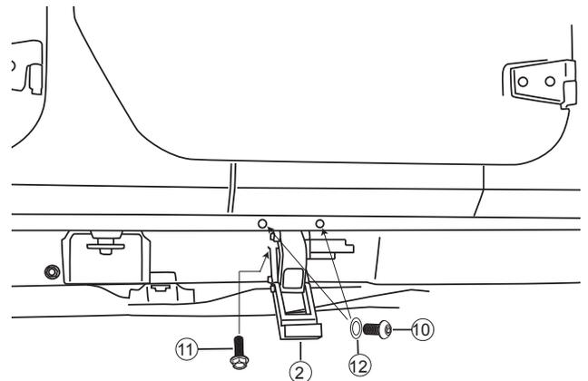
Torque fasteners to 16 ft-lbs. (22 Nm)
