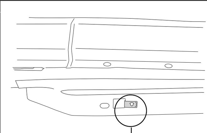
**4** Install U nut under vehicle, middle of front door for front motor linkage as shown. (Some vehicles with factory steps may already include this u-nut)
