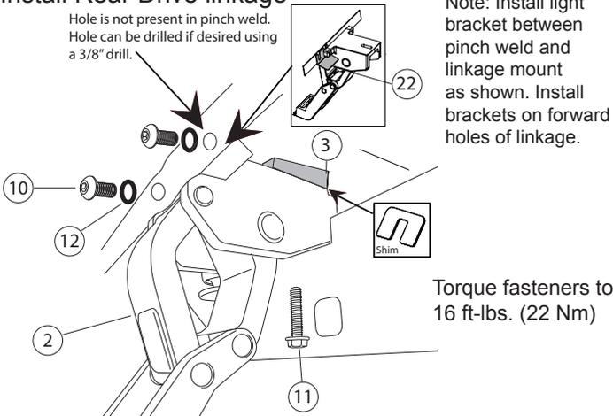
Note: Install light bracket between pinch weld and linkage mount as shown. Install brackets on forward holes of linkage.
