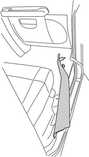
Lift carpet. Slit rubber grommet and pass trigger wires through grommet in floor into passenger compartment.
