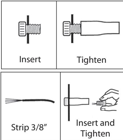
Use Posi-Tap connectors to connect Power Step trigger wires to like colored wires in the factory system as shown: Violet/White wire in loom coming from front door, Violet/Yellow and Violet/Grey in main loom in door sill. **Note: For door removal attach posi tap on chassis side of door harness. See Step 17 for plug access.**
