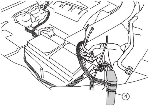
Attach wire harness to controller (make sure connector locking tabs fully engage). Mount controller with the two 11" tie wraps to factory conduit, just forward of battery.
