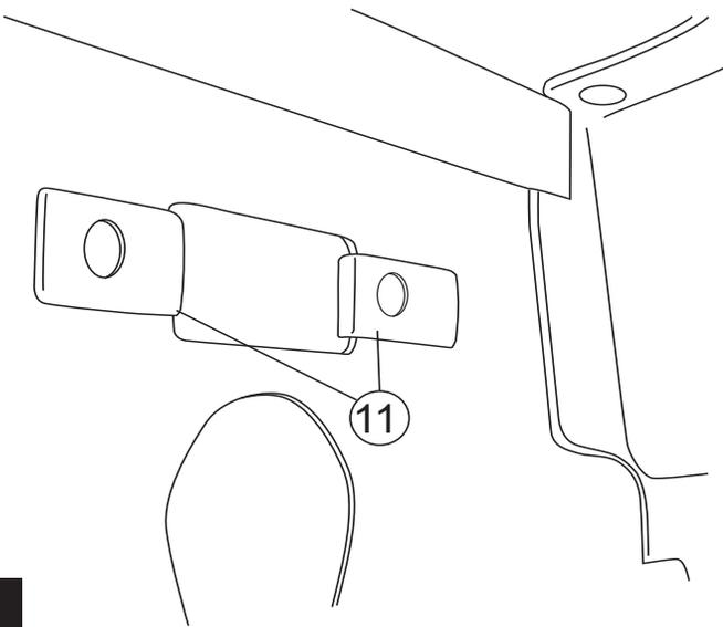
Torque fasteners to 16 ft-lbs. (22 N m).
