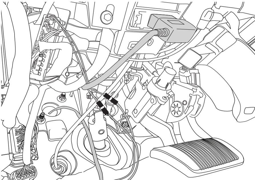
Note: To remove 2 pin connector (if needed) once plugged in, use a tool to push down clip as shown below.
