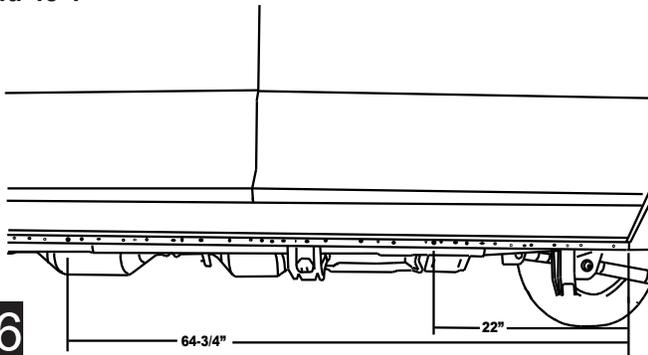
Drill a 9/32" hole through the pinch weld at marked locations. Deburr all holes. After drilling apply paint to holes to prevent rusting.
