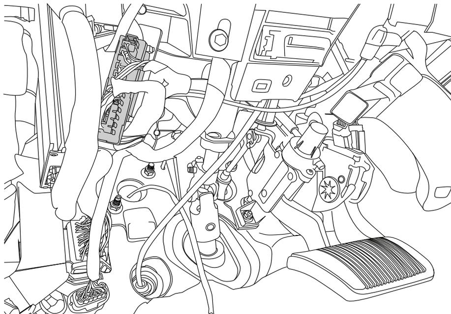
Plug 2 pin plug into the Green Connector Block. Use supplied Posi-Lock connectors to attach the Plug and Play module to the Harness. Attach Matching colors on the harness to the wires on the module. Plug in module to the OBD II port on the vehicle. Secure harness with supplied tie wraps.
