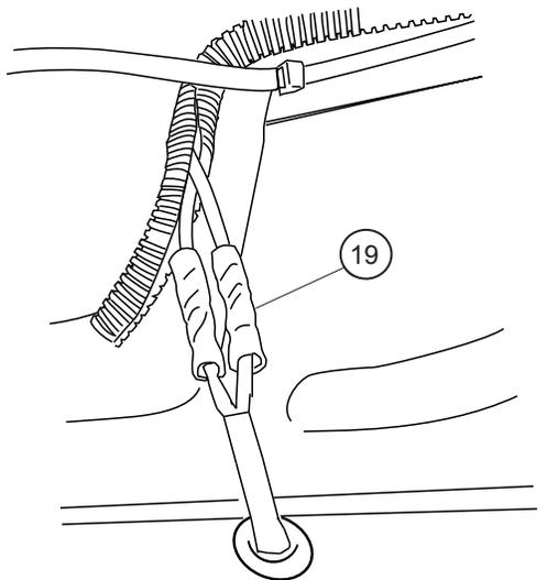
Close and wrap with conduit and electrical tape. Secure all loose wires with cable ties, with lamp wires pulled upward to avoid any wire snagging.
