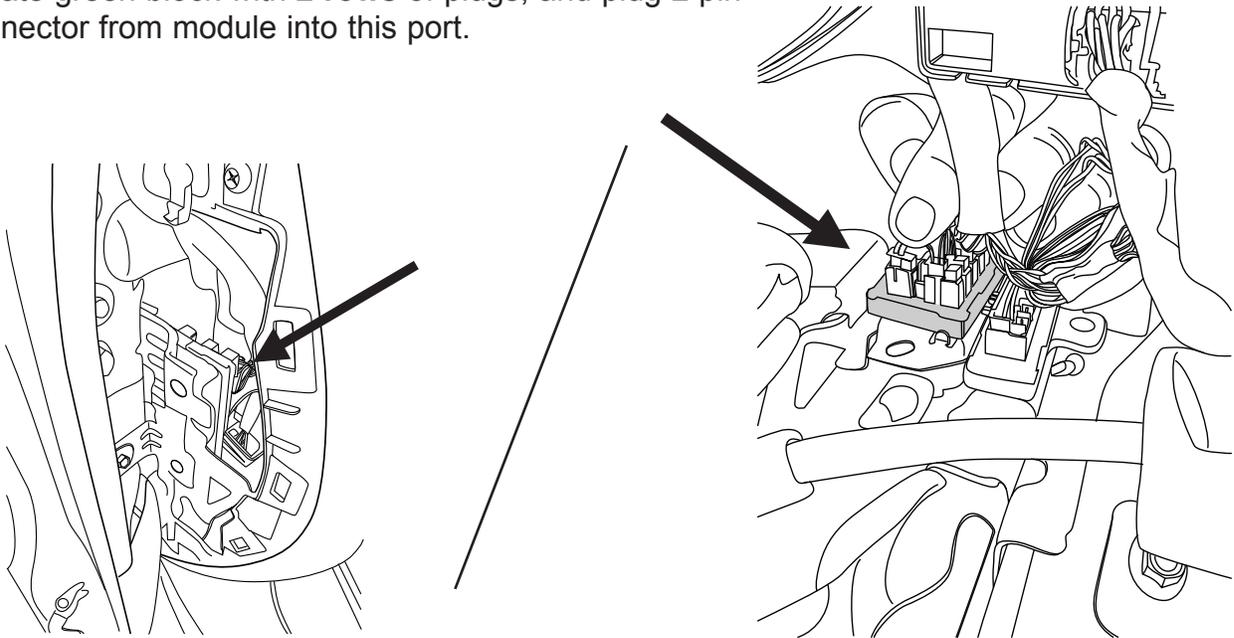
**Note:** It's best to reach from both sides when installing 2 pin plug. Any open port on green plug can be used.
