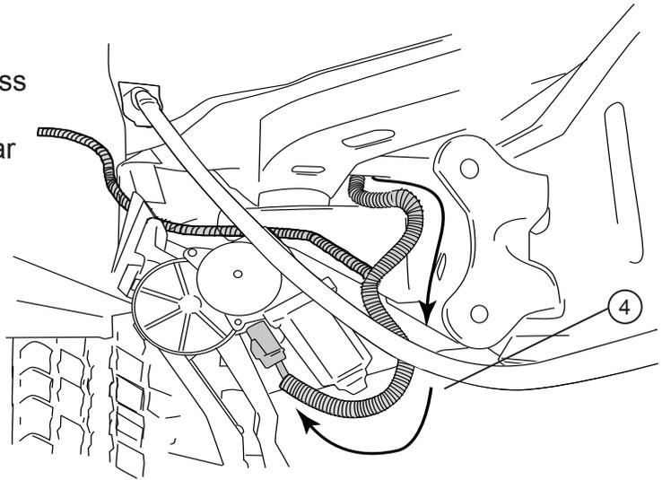
On Passenger Side, run Wire Harness leg down and along underside of the vehicle floor and frame to front Drive Linkage. Connect harness to motor and secure harness with tie wraps. Route remainder of wire harness towards rear linkage assembly for LED lights
