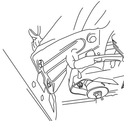
If crash bracket is not present use supplied spacer in place of bracket. Spacer can be inserted after linkage is up into position. Spacer will be held in place by drilling and pop riveting into place. **Rivets will be installed in step 42 & 43.**
