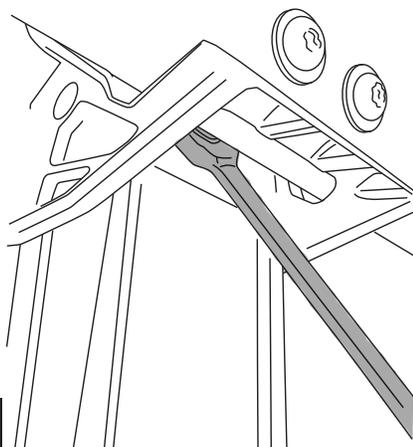
Using a T27 Torx driver torque bolts to 6 ft-lbs.
