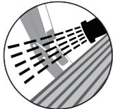
**Maintenance:** In adverse conditions, debris such as mud, dirt, and salt may become trapped in the running board mechanism, possibly leading to unwanted noise. If this occurs, manually set the running boards to the deployed position and flush the front and rear hinge arms with a high-pressure car wash wand.
