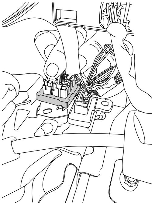
Note: To remove 2 pin connector (if needed) once plugged in, use a tool to push down clip as shown below.
