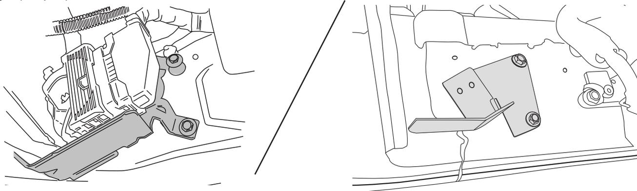
Locate mounting points. First and last set of studs on the inner sill. Motor linkage mounts towards the front of the truck and Idler towards the rear. Driver side shown below.
