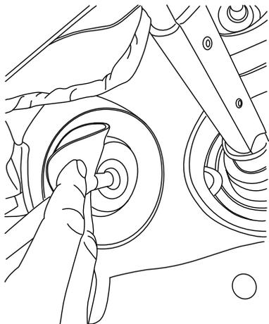
Plug OBD (7 ) to port, tuck wires up and away to prevent snagging when entering and exiting the vehicle.
