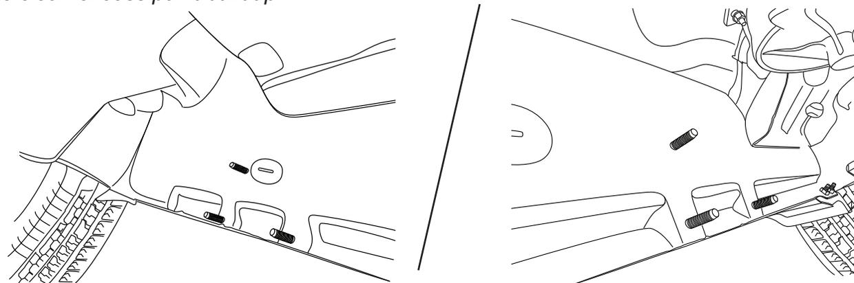
Mount drive and Idler linkage assemblies using supplied conical washer nuts (11) use a 13mm socket or wrench to tighten. Repeat for passenger side. Make sure linkages sit square, fully resting on studs before tightening. Torque to 16ft-lbs (22Nm).
