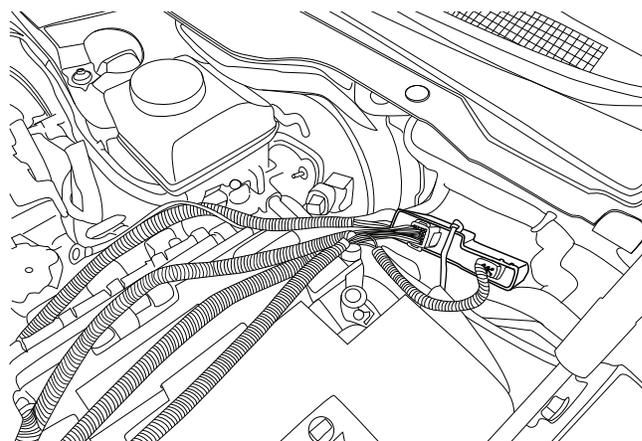
Connect red power lead to battery. Connect black ground lead to 13mm bolt outside of fender wall.
