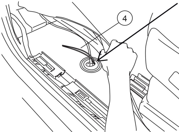
Route the two trigger wires towards the rear of the vehicle above the body mounts, and up through the hole made in the rubber grommet in the previous step. Secure harness with supplied cable ties.
