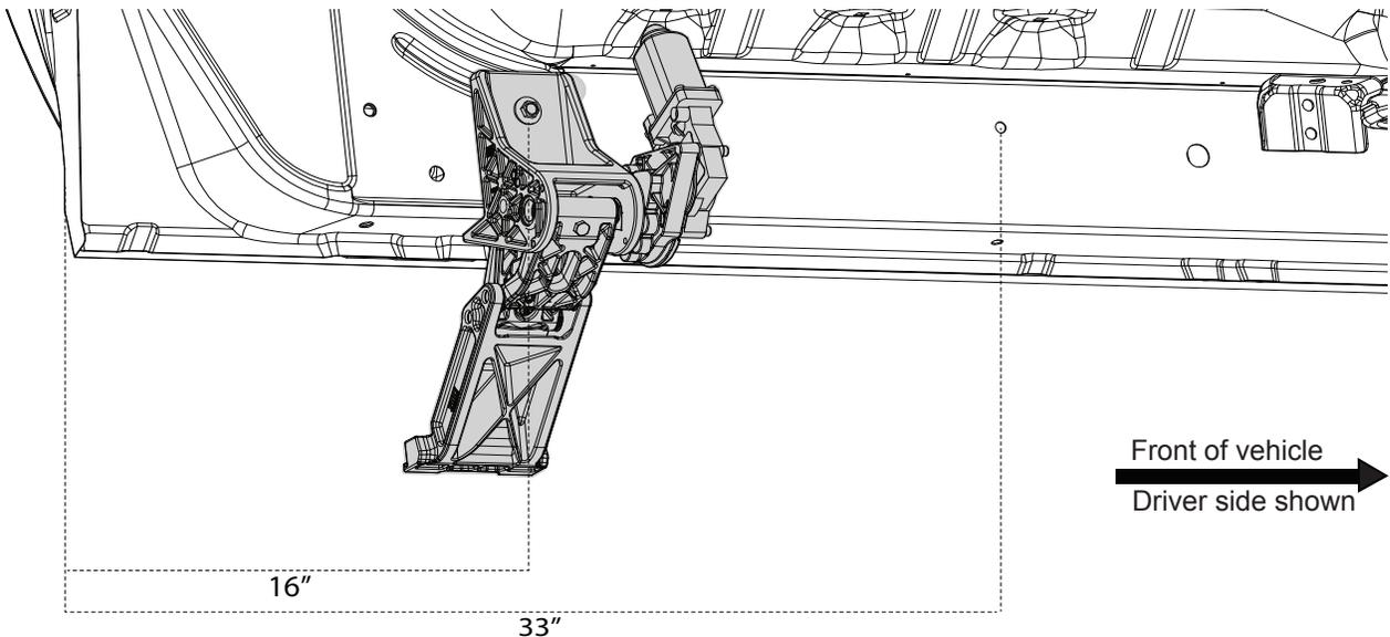
Assemble the motor to the linkage like the picture before installation shown on page 2. **Position the motor so the linkage is in the mid extension position.** This way the lower bolt can still be installed.
