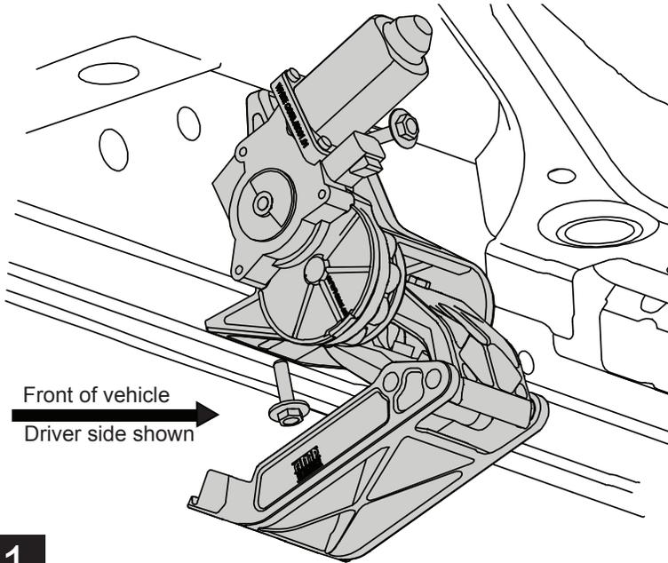
Install motor linkage B in the the First mount position at the front of the truck on the Driver side, using the bolts supplied (12). All plastic or rubber hole plugs need to be removed that are next to the linkage mounts. Torque fasteners to 16 ft-lbs. (22 N m).
