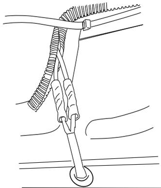
Using supplied butt connectors(15), connect the lamp wires. Red to Red, Black to Black. Once Crimped use heat gun to shrink tube.
