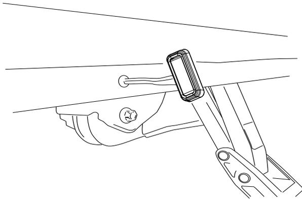
Insert grommet(16) into drilled holes. Insert lamp(9) wires through the grommets. (Silicon lube will help wires slip through grommets)
