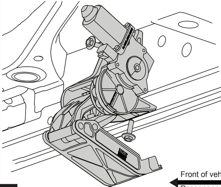
Install motor linkage A in the the First mount position at the front of the truck on the Passenger side, using the bolts supplied (12). All plastic or rubber hole plugs need to be removed that are next to the linkage mounts. Torque fasteners to 16 ft-lbs. (22 N m).
