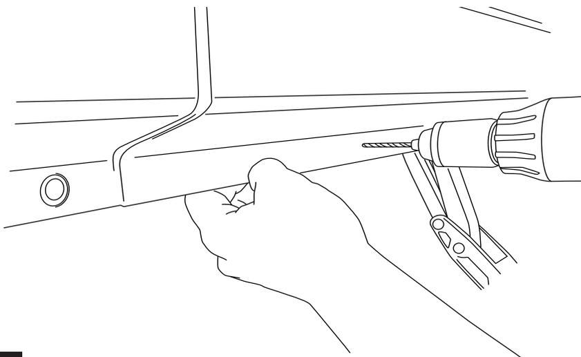
Center punch and drill a 1/8" pilot hole then drill a 19/64" hole through the pinch weld at marked locations. Deburr all holes. After drilling apply paint to holes to prevent rusting.
