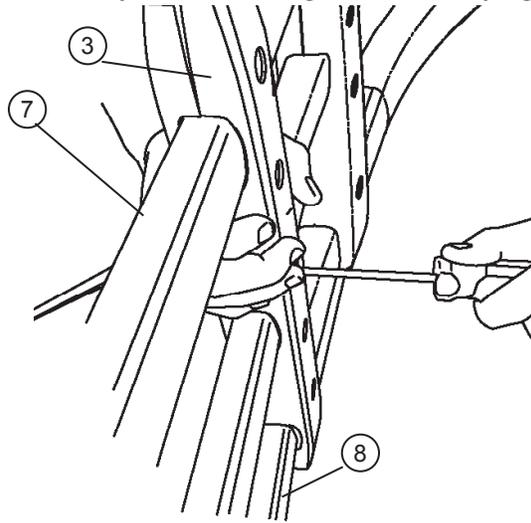
**NOTE:** Do not over tighten as this may strip out. Fastener will reach a noticeable stopping point.
