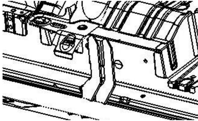
**Step 4** After final adjustment tighten all the lower mount first then the upper mounts.
