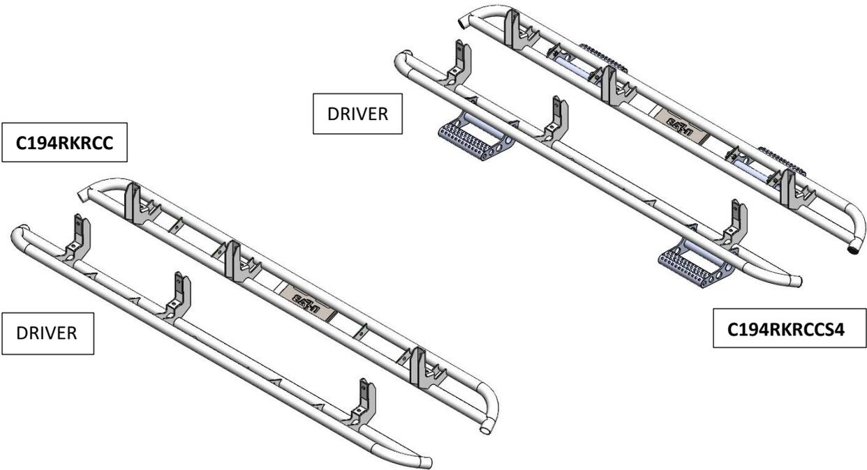
**Step 2** Carefully raise the RKR rail up into position aligning the mounting brackets with the factory-threaded holes. Beginning with the center bracket start one of the supplied M8x30mm Hex bolts in the upper mount and finger tighten. This will allow the rail to be suspended while you start the remainder of the hardware.
