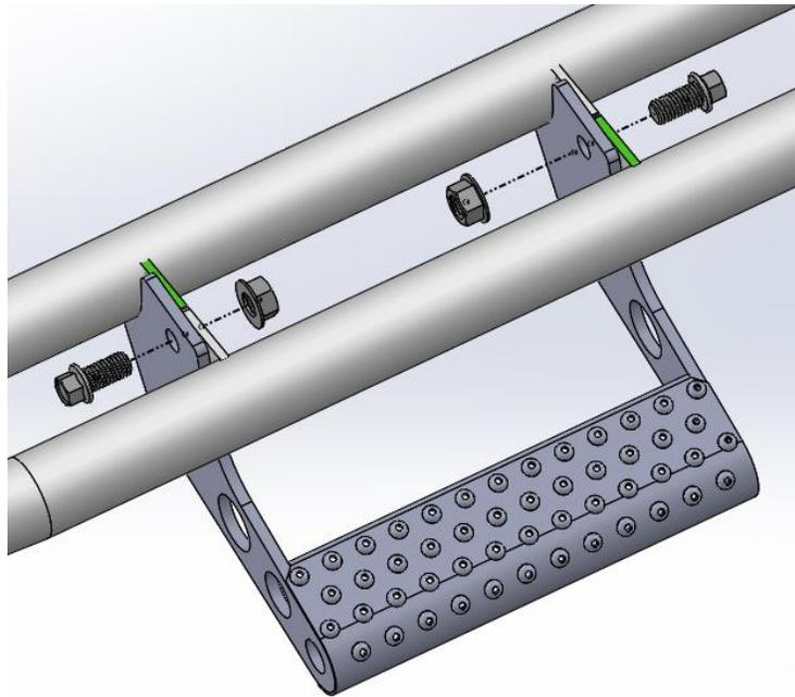
**Step 2:** Torque bolts to a target torque of 40 ft.-lbs. / 54Nm
