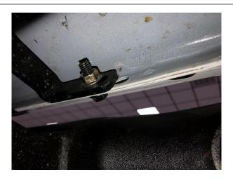
**Step 8:** Begin tightening the lower attachment points starting with the rear bracket working your way up to the front bracket. **( 20ft/lbs )**
