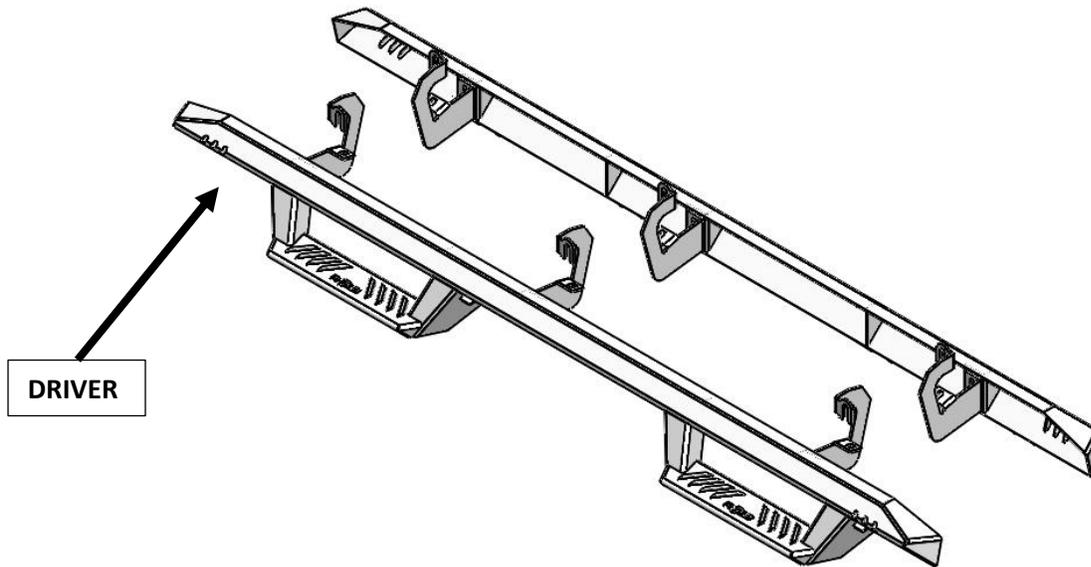
**Step 2:** Install three rocker panel brackets to the attachments points located on the backside of the channel using the supplied 3/8" x 3/4" carriage bolts and 3/8" flanged nuts. Leave finger tight for now.
