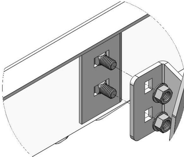
**Step 3:** With the correct step placed on each side of the vehicle, take note of where the brackets are located. Look under the vehicle and locate the factory supplied mounting positions. **NOTE:** *Some vehicles require the use of supplied clips and nuts.*
