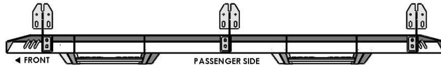
**Step 3:** locate the six sets factory mounting hex holes (3 on each side of the vehicle). These are positioned on the vertical sides of the floor pan beneath the doors, with one set of holes each in the front, middle, and rear of the vehicle cab.
