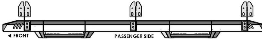
**Step 3:** Locate the six sets factory mounting hex holes (3 on each side of the vehicle). These are positioned on the vertical sides of the floor pan beneath the doors, with one set of holes each in the front, middle, and rear of the vehicle cab. **NOTE: If your model is equipped with the M8 threaded inserts skip step 4.**
