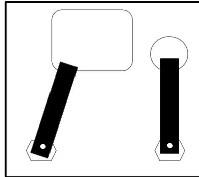
Some modes may require drilling a 1" hole in the rear attachment point in the body panel to extend the threaded clip to the opening.
