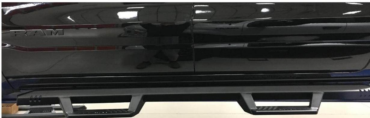
**Step 8:** After final adjustment, tighten all rocker panel brackets to 30 ft./lbs.
