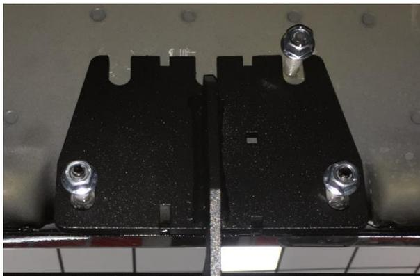
**Step 6:** Next, adjust the step assembly up/down and front/back to level out the step rail with body panel and then tighten step to brackets at 30 ft. /lbs.
