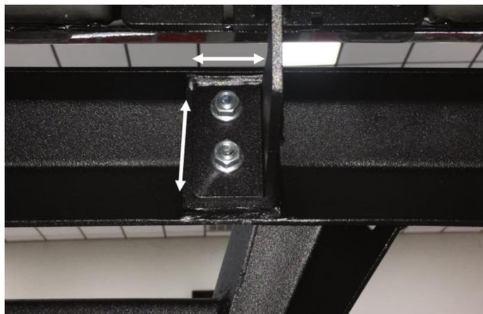
**Step 7:** Adjust the step rail to where you have approximately  $\frac{1}{4}$ " gap between the body of the vehicle and the top of the rail.
