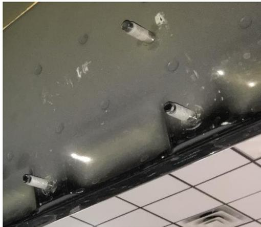
**Step 5:** An additional person is recommended for this step. Carefully install the step assembly to the three factory attachment points using the provided M8 flanged hex nuts. Leave finger tight for now.
