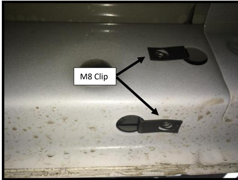
**Step 7:** Carefully raise the nerf-step into position aligning all brackets with the three mounting holes. Insert all six M8 X 25mm HC bolts. Use the smaller 3/8" washers for the bottom bolt and the larger Fender washer for the top bolt and hand tighten only.
